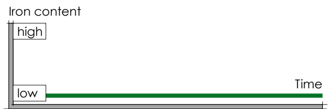
The Recyclean method: Constant iron content under 1 g/l < 1 gFe/l.
